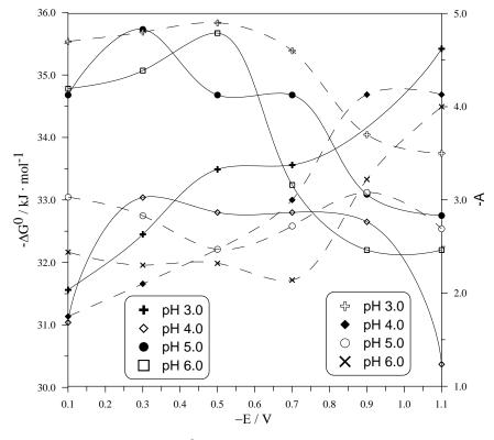
Fig. 8. The value of adsorption free energy  $\Delta G_F^0$  (solid line) determined from the Frumkin isotherm and the value of parameter A obtained from linear tests of the Frumkin isotherm -A (dotted line) for the system containing adenine in the acetate buffer with varying pH
