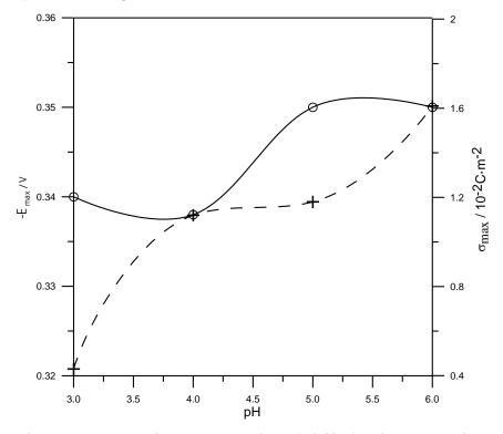
Fig. 6. Correlation between maximum adsorption potential  $E_{max}$  (solid line) and maximum adsorption charge  $\sigma_{max}$  (dotted line) determined for various adenine concentrations in the acetate buffer with varying pH
